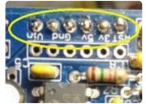
**Repair:** This condition can usually be repaired by placing the tip of the hot iron at the base of the joint until the solder flows to cover the pad.
